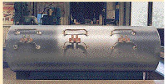
8. The furnace is wired for three zones. Note the slack in the braids.
