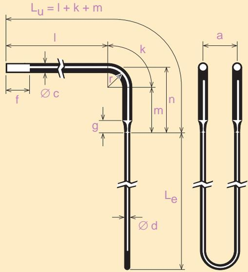
Fig. 7 Element bent 90° at the terminals.
