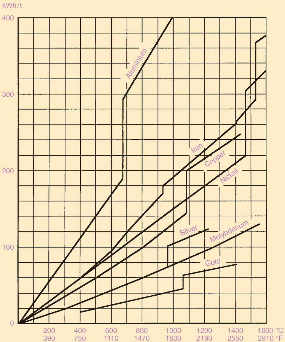
Fig.74 Average theoretical heat storage in kWh per metric tonne for some common metals.
