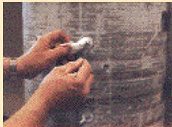
5. After the two half-shells are bolted together, raise the furnace to an erect position. Seal around the terminals with ceramic fibre wool. Do not pack too tight. Be careful not to create stress in the terminals.
