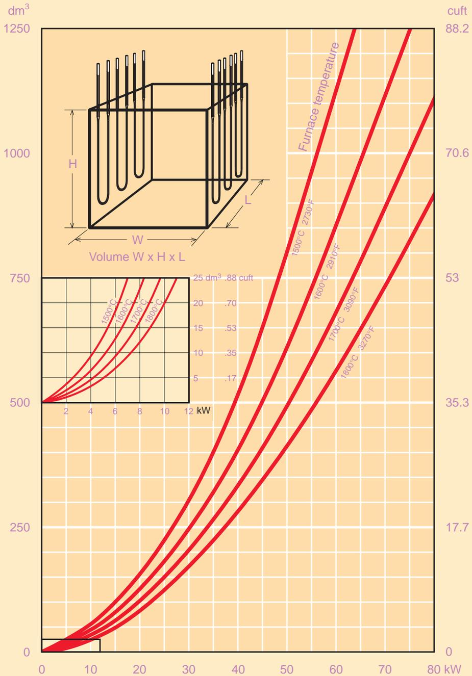
Fig. 52 The approximate power at a given chamber volume for a ceramic fibre lined furnace. For a brick lined furnace the power is normally about 25 % higher.
