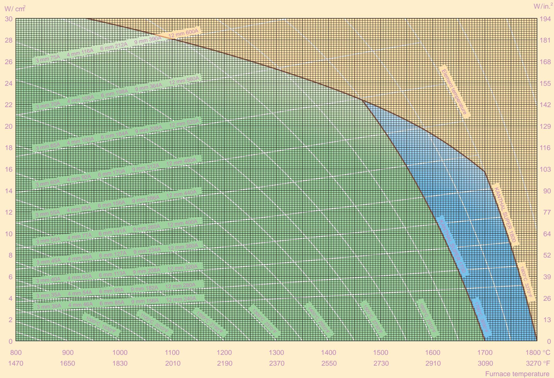
Fig. 27 Temperature — loading diagram for KANTHAL Super 1700 (green) and 1800 (blue).
