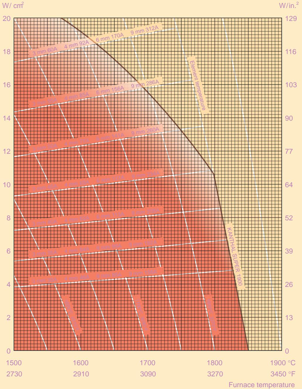
Fig. 28 Temperature — loading diagram for KANTHAL Super 1900.
