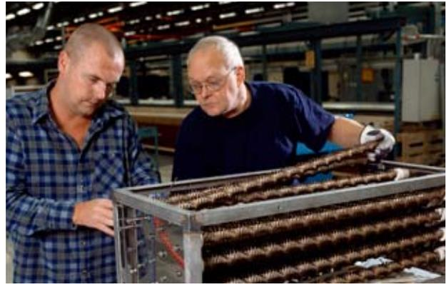
The heating elements are made in the form of a special spiral and mounted on ceramic tubes
