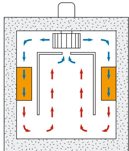
Baffles direct the recirculating air/gas through the heating elements
