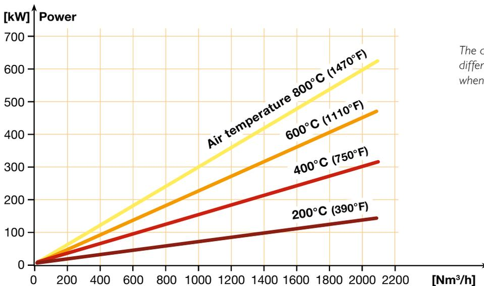
The diagram shows the needed power for different air/gas temperatures and flows when starting from room temperature
