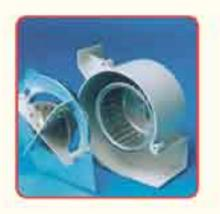
9 Heater with integrated Venturi plate completes the blower and mounts easily to the blower housing. Client needed well mixed warm air but had a temperature sensitive material near the exhaust. So, we designed the heater to almost nest into the impeller for max. efficiency and mixture. Heater overtemp device is configured to stop blower motor.
