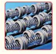
Food service cooker. Heater designed to fit narrow slot for maximum heat transfer and minimal product size. Circuits are canted to turbulate the air for maximum efficiency. Cuts cooking time by 40% and browns product too. Passes 2500 volt hi-pot at 1000F.
