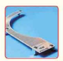
5. Circuit board mounted heater for product where there was 'no space' for a heater and the discharge temps had to be thoroughly mixed and even. Heater designed to fit in the scroll of the blower in an aerodynamic low profile so that the performance of the blower is not affected.
