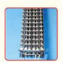
4. 15kw Convection heater for Food Service ReThermalization Cart. Designed for ruggedness and to bring 60 lbs. of frozen meals to 140F in 20 minutes.
