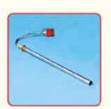
3. Small 187" diameter heater for assembly into 0 clearance probe in a scientific instrument. Precision heating of gas stream is critical. A custom RTD has been designed into this small package. Heater integrates air tight seal inside probe.
