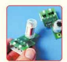
1. Miniature heat torch mounted on circuit board. Had to fit 1" space and focus hot air precisely to help blow mold pouches on blood analyzer. Has to heat ambient to 390F in 3.5 seconds. Thermocouple is built in.
