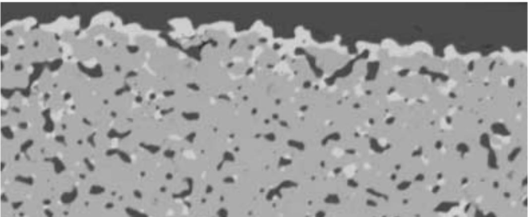
Fig. 3 Microstructure of a KANTHAL SUPER element. Grey =  $\text{MoSi}_2$ . White =  $\text{Mo}_5\text{Si}_3$ , Dark =  $\text{SiO}_2$ .
