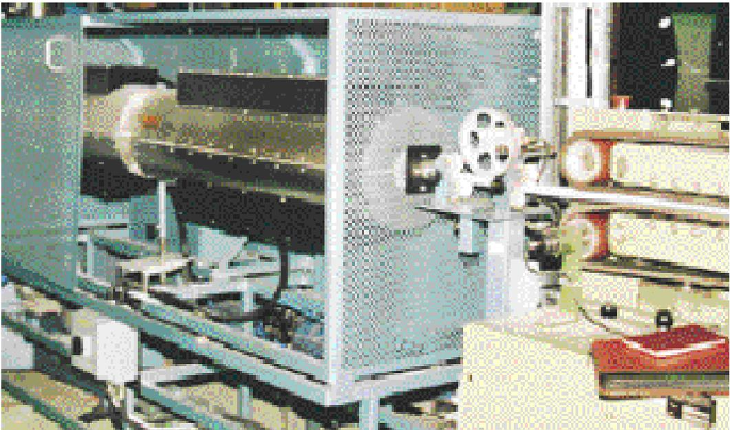
Fig. 21 SUPERTHAL tube furnace for materials testing and as IR-heater at plastic pipe manufacturing
