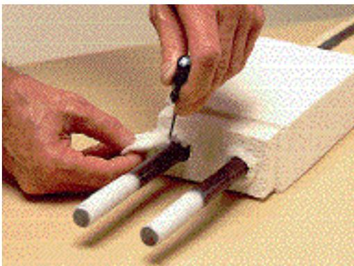
4. After packing heavy-duty ceramic fibre loosely into the recesses of the terminal holes
