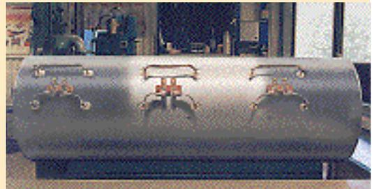
8. The furnace is wired for three zones. Note the slack in the braids.
