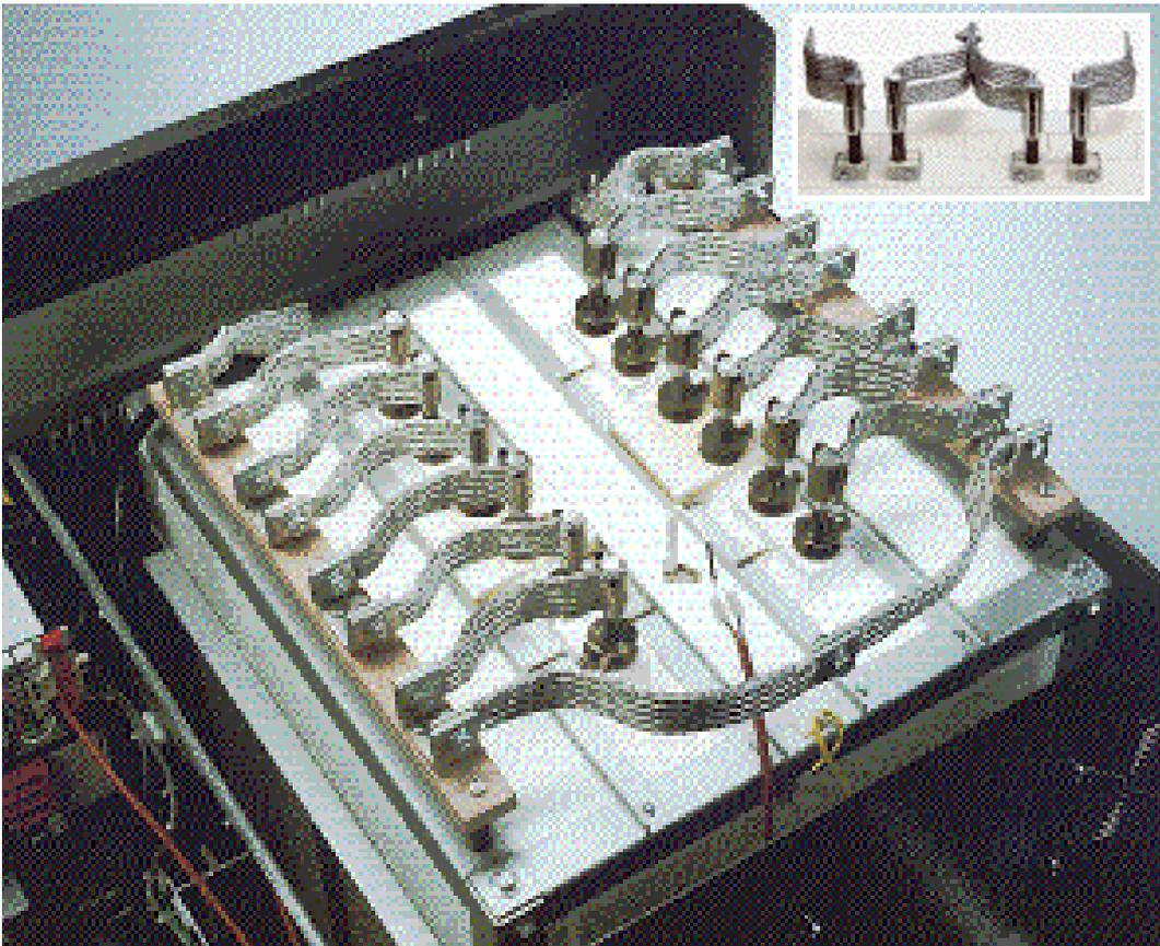
Fig. 45 KANTHAL SUPER elements connected to busbars.
