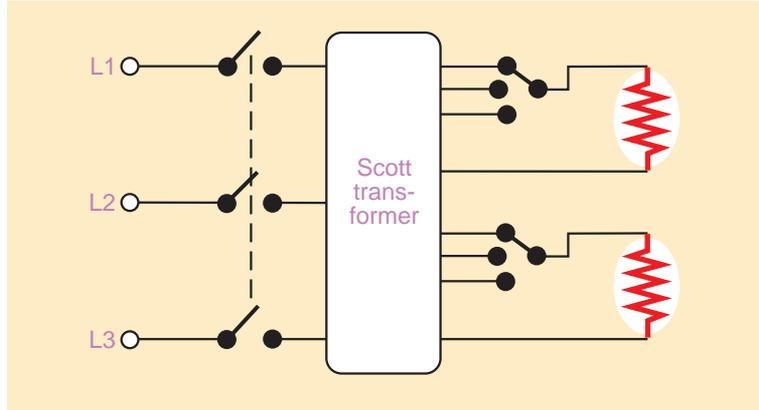
Fig. 63 Application with on/off control and tapped transformer.
