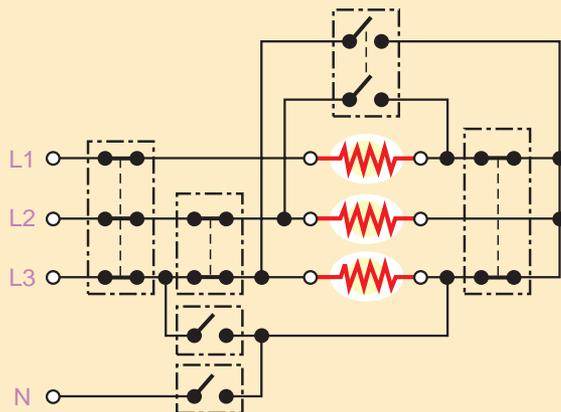
Fig. 61 Wiring diagram for KANTHAL SUPER elements directly star-connected to line voltage.
