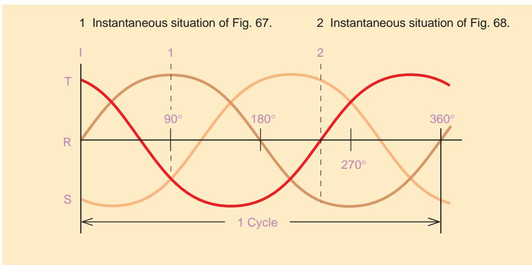
Fig. 65 Sine curve variations in a three-phase system.
