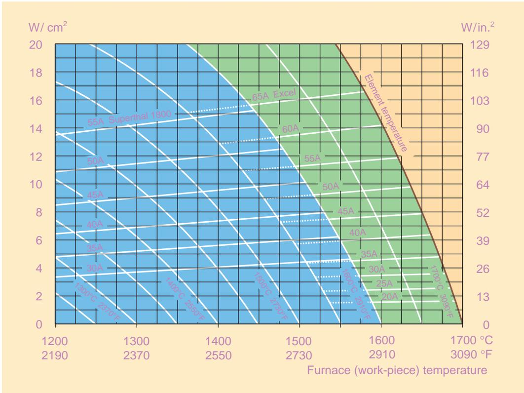
Fig. 17 Temperature — loading diagram for SUPERTHAL.
