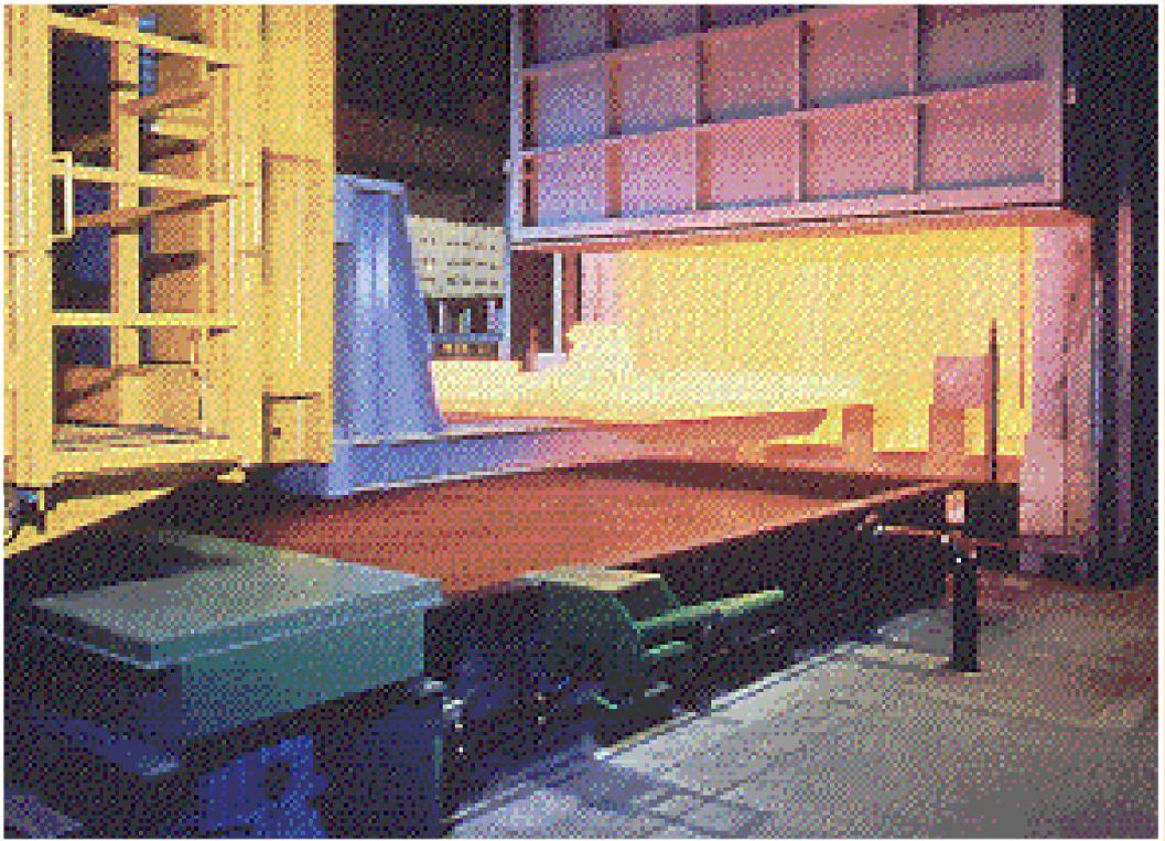
*Fig. 71 Automatic hardening line heated with KANTHAL SUPER elements located in the floor, in the door and along the three walls.*
