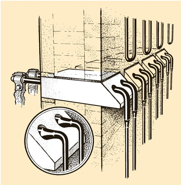
*Fig. 32 KANTHAL SUPER elements, with terminals bent 90°, installed in a brick lined furnace.*
