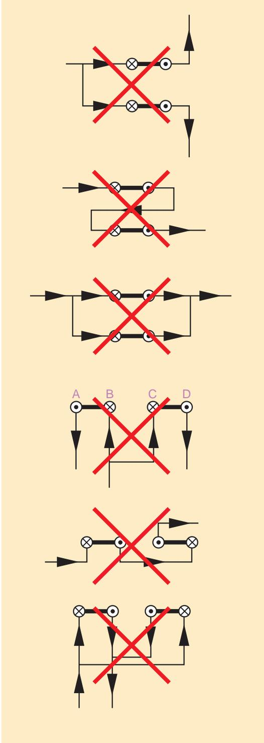
Fig. 66 Examples of correct and incorrect connections.
