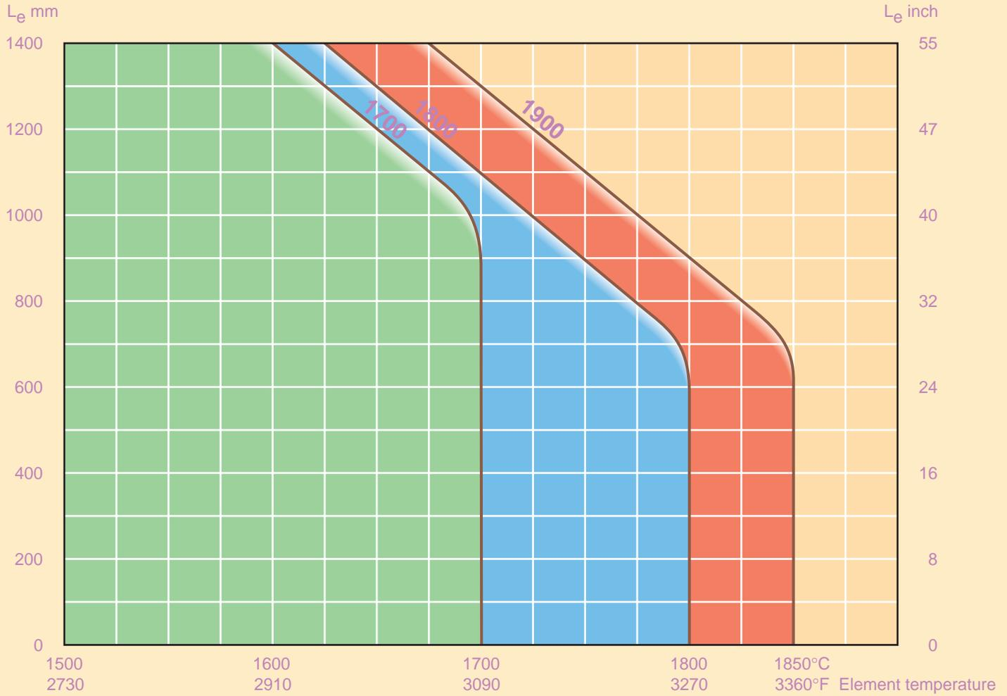
Fig.12 Maximum recommended heating zone lengths for vertically suspended 6/12, 9/18 and 12/24 mm elements.
