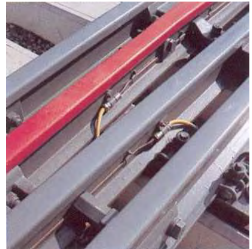
Heating element in springy moving frog UIC 60 - 10000/4000 - high-speed line Madrid - Seville
