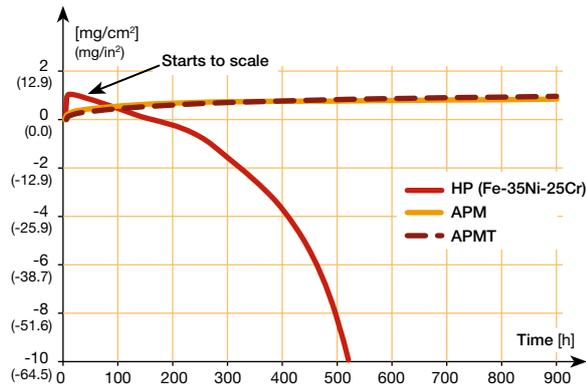
Figure 3b Sample weight gain – 1100°C (2010°F).
