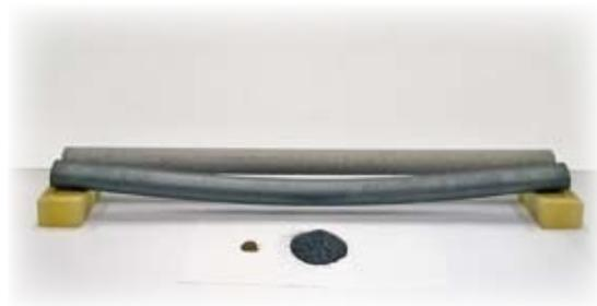
Figure 4 Comparison of APMT Tube vs. Fe-35Ni-25Cr (after 2300 h at 1100°C (2010°F)). The FeNiCr tube is severely contaminated with oxide flakes.
