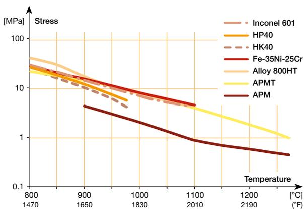
Figure 1 Creep rupture strength – 10 000 h.
