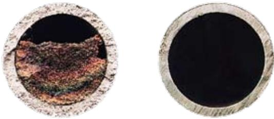
Figure 6 Comparison of carbon build-up in a strand annealing furnace, NiCr (left) and APM/APMT (right).
