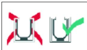
Allow space for expansion between crucible and furnace lining/cover.
