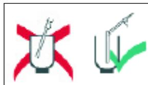
Ingots should be loaded carefully into the crucible using tongs.
