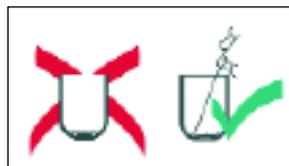
The crucible must be emptied before switching off the furnace.
