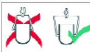
Lift-out tongs should hold crucible on it's lower third and fit evenly on both sides.
