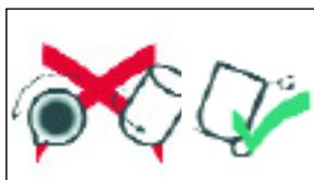
Do not roll crucibles. Move using a sack truck with padding.
