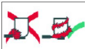
The flame path must be tangential to the crucible.
