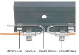
Electrolux point-heating elements are attached to the rail foot using special clamping yokes made of corrosion-resistant chrome-nickel steel. The clamping pressure is chosen so that optimal heat transfer is guaranteed. Inevitable lateral expansion during heating can occur without affecting operation.
