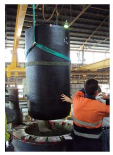
Fig. 3. A cylindrical crucible is installed in an induction furnace.
