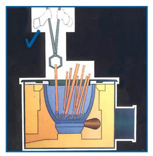
Fig. 5. Crucibles that provide impact resistance are often selected for furnaces that are manually charged with ingots and other solid materials.
