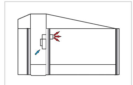
Pig Heaters are designed to be located within a pig building by blowing heated air into those rooms within the farm where it is needed for the pigs, in particular, the Farrowing and Weaning Houses. Each of the drawings above illustrates typical mounting arrangements for the unit, also highlighting the flexibility in
