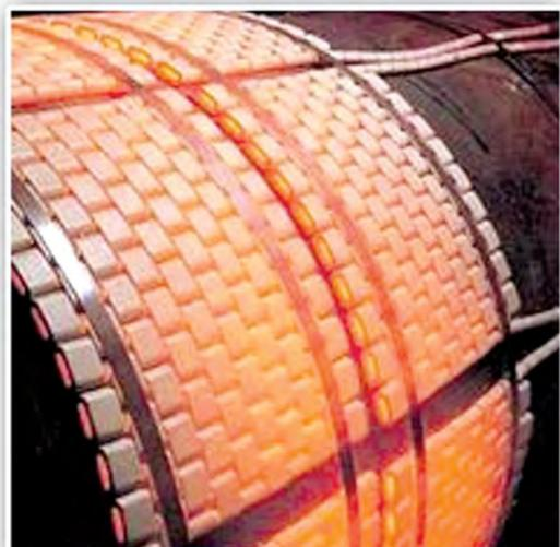
Flexibility of electrical heaters enables the application of electro-resistant heating at heat treatment of all kinds and forms of welded joints.
